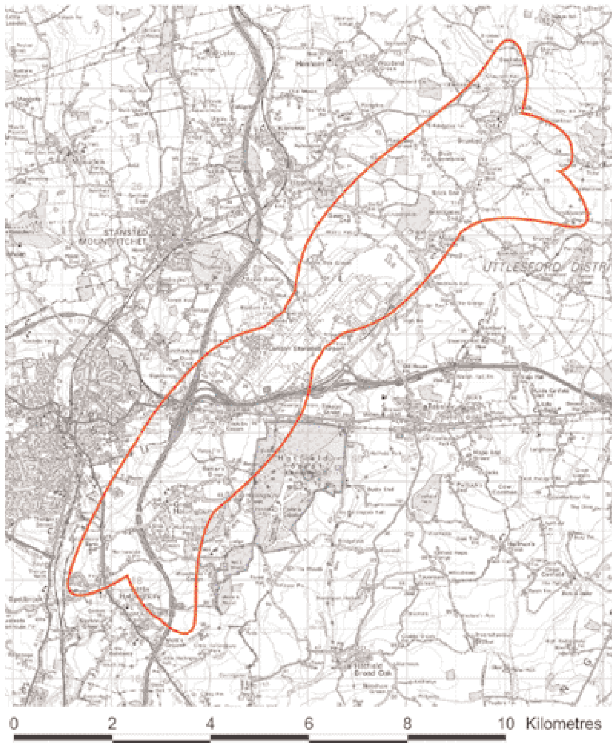
Possible insulation scheme boundary at Stansted based on the envelope of the 90dBA SEL footprints for MD-11 departures
