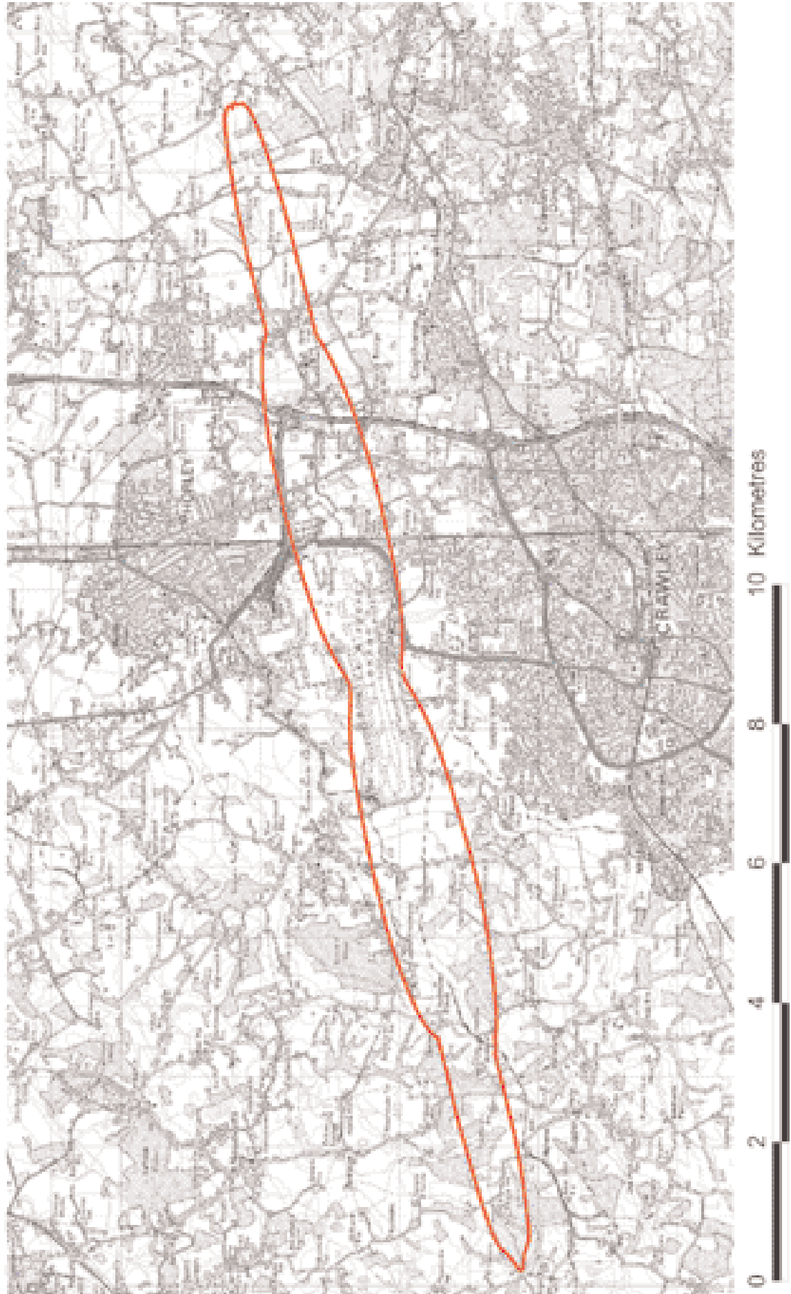
Possible insulation scheme boundary at Gatwick based on the envelope of the 90dBA SEL footprints for Airbus A300 departures and Boeing 747-400 arrivals
