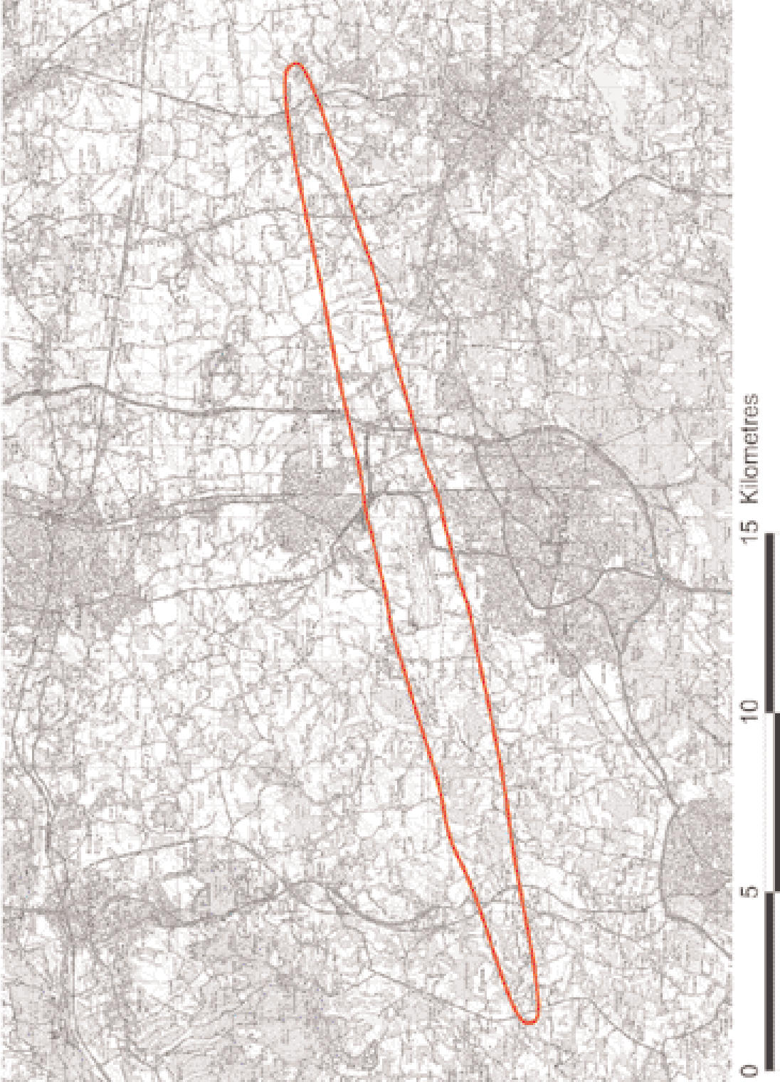
Gatwick 2300-0700 50dBA Leq contour consistent with noise abatement objective set out in chapter 4
