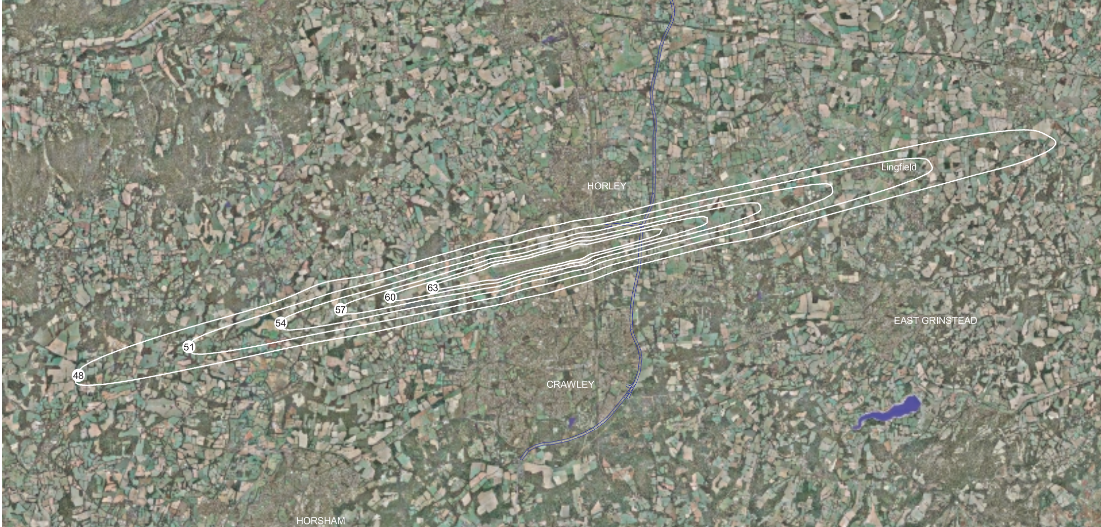
Figure 10: Gatwick October 2002 – October 2003 average mode L_{\text{night}} (6.5 hour) contours (48-63dBA) assuming maximum quota usage
